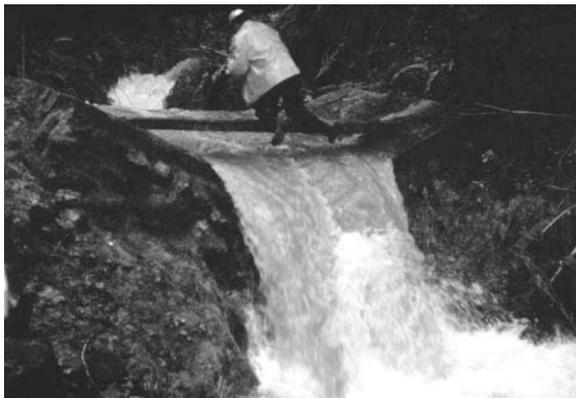
**Figure 3** Early estimates of sediment flux from drainage basins relied on sampling suspended sediment over a range of flows and integrating results over time, a technique that provided sediment yield data for which extrapolation back in time was uncertain. Photograph circa 1960 of suspended sediment sampling from the H.J. Andrews Experimental Forest (Photo AAB-057 used with permission of H.J. Andrews Experimental Forest).
