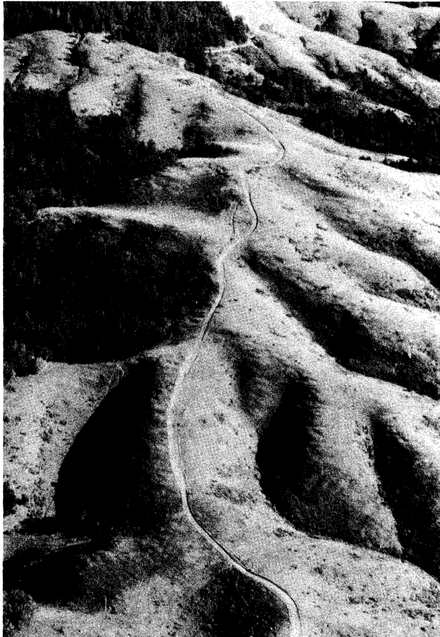
Figure 17.1 View of unchannelized basins on hillslopes in Marin County, California. Note tributaries or subhollows within larger unchannelized basins.
