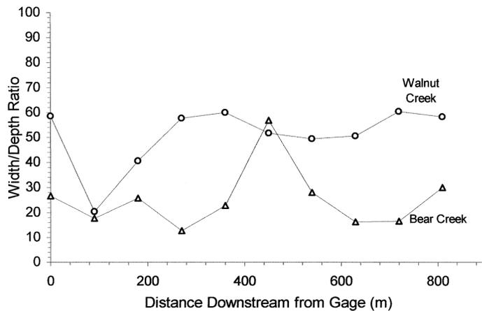
Figure 9. Channel width/depth ratios measured along Walnut Creek (circles) and Bear Creek (triangles) just below the USGS stream gage stations. Walnut Creek has a shallow channel that increases in width downstream, typical of alluvial-stream channels, whereas Bear Creek is more deeply incised.
