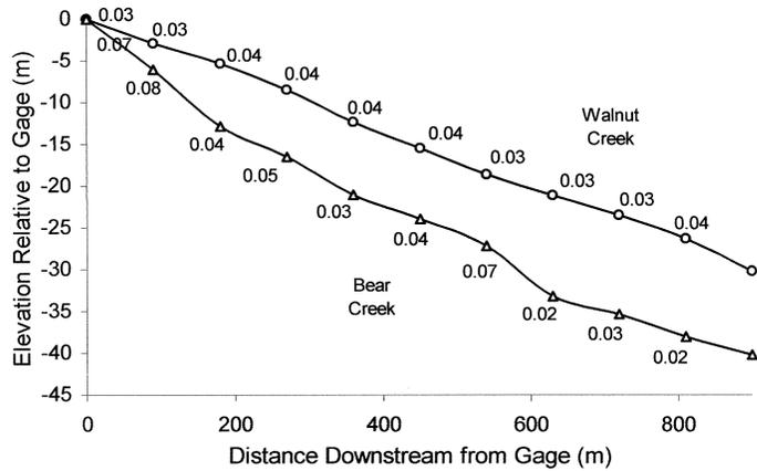
Figure 8. Longitudinal stream profiles for Walnut Creek (circles) and Bear Creek (triangles) immediately below the USGS gage stations. The measured channel gradient is displayed for select points along each profile.
