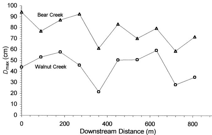
Figure 10. Sediment caliber for Walnut Creek (circles) and Bear Creek (triangles) based on the five largest clasts sampled.
