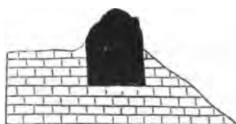
FIG. 21.—Ideal Cross-section of a Flat-bottomed Dike.
