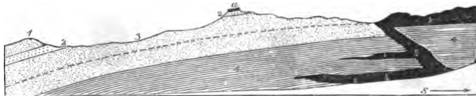
FIG. 23.—Section shown in a northward cañon of Mount Holmes. a , Vestige of Trachyte sheet. b b b , Trachyte sheets. c , Trachyte dike. 1, Gray Cliff Sandstone. 2 2, Purple Sandstone. 3, Vermilion Cliff Sandstone. 4, Shinarump Shale.
