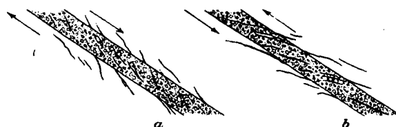
FIGURE 3.—Ideal sections of faults and of subsidiary slickened partings, to illustrate the relations of the attitude of the partings to normal faults (a) and reverse faults (b)
